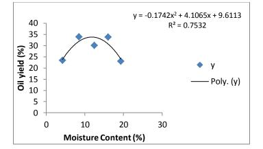
The above graph of oil yield against moisture content shows the line of best fit for the given data in table 3. The coefficient of determination,  $r^2$  is 75.3%, which is an indication that the oil yield for Soursop seeds can be reliably related to its moisture content by the polynomial equation below
