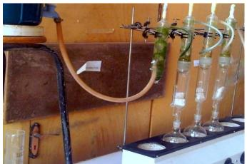
Fig.1 the Soxhlet extractor set up in series for three extraction processes.
